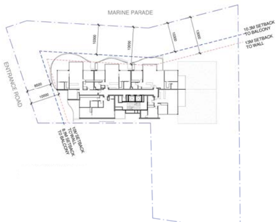
FIG. 42 TYPICAL TOWER LEVEL SETBACKS
